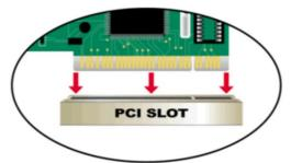
*Note:* To avoid static electric charges, please touch an unpainted screw on the outside of the power supply before installing or working with the DFE-528-TX.
